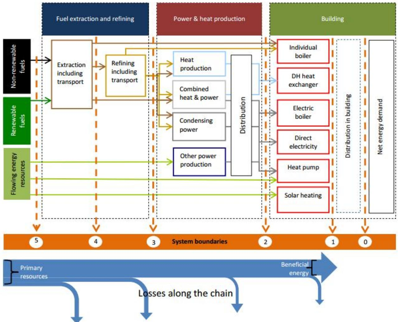
Figure 6: Illustration of alternative system boundaries and of losses along the energy chain from primary resource to heating of a building. (Source: IVL, Ecoheat4cities Work Package 2 Green Labelling Criteria, 2011)
