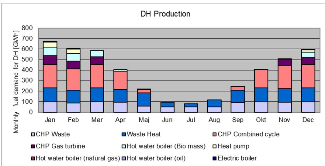
Figure 3: Example of DH production and fuel sources.
