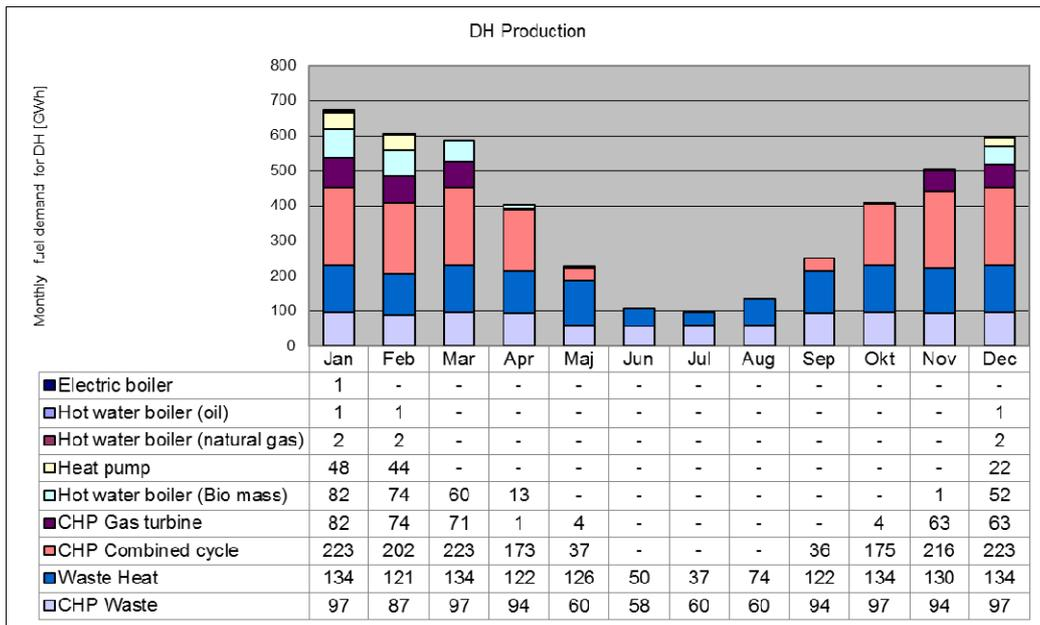
Figure 5: DH production profile with supply to absorption chillers for DC.
